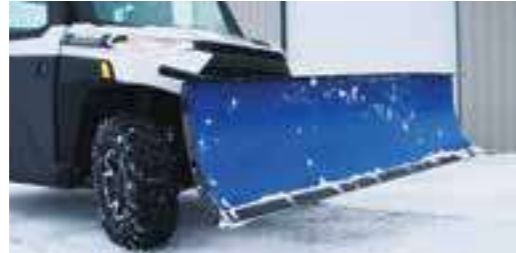
PLOW IS AUTOMATICALLY RAISED WHEN SHIFTING INTO REVERSE
